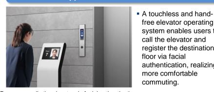
free elevator operating system enables users to call the elevator and register the destination floor via facial authentication, realizing more comfortable commuting.
